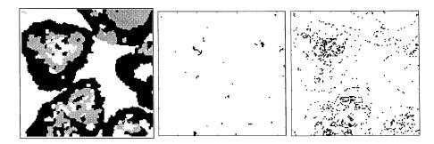
Fig. 9. Segmentation stability. The left image is a segmentation result. Binary images show pixels with a non-zero probability of label change in a set of segmentations started by different random initialization of the initial labeling algorithm. The image in the middle corresponds to the classifier-based segmentation and the rightmost image to the probabilistic relaxation.
