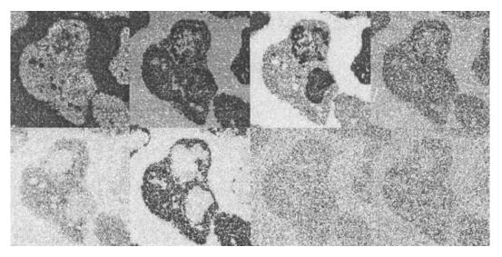
Fig. 2. Multi-spectral image with eight bands acquired by SEM/EDX method.
