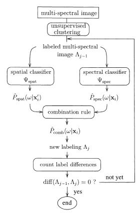
Fig. 1. The segmentation algorithm.
