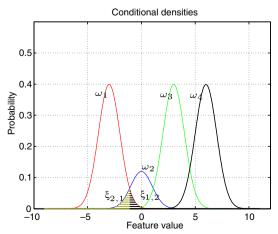
Fig. 1. Probability density functions for the four-class example with known distributions. Two operating points are shown, with the left plot involving equal output weighting, and the right with a higher  $\phi_2$  and lower  $\phi_1$ .
