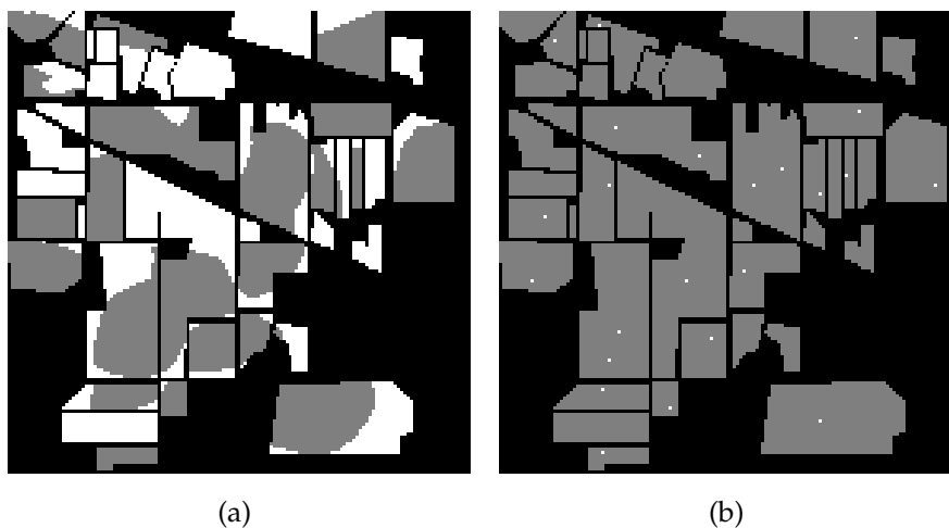
Figure 5.7: Classification results using 24 spectral/spatial features and 23 selected training samples. (a) representation of misclassified pixels in white and (b) training samples shown in white. Error rate was 0.41.
